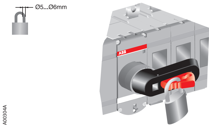
Fig. 6-8 Locking manual operation
