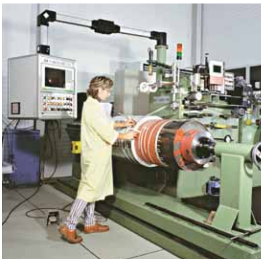
winding an HV coil in strip
